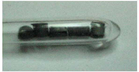
Fig. 5. \text{Be}_{12}\text{Ti} specimens sealed in the quartz tube delivered to High Flux Reactor, Petten, Netherlands (1/4 of the page).
